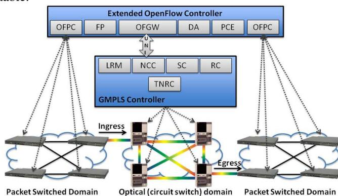
Figure 3. Integrated GMPLS-OpenFlow control plane.
