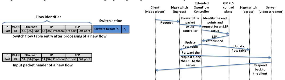
Figure 4. a) Extended flow table entry in the ingress switch (left) b) Timing diagram for a use-case (right).
