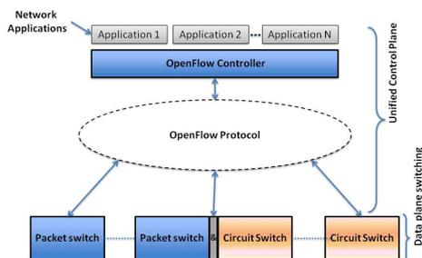
Figure 2. A unified control plane based on OpenFlow protocol, controller and network applications.
